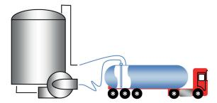
Some vehicles are designed with 'dip-pipes' to accommodate top-discharge. The same possibilities exist as for bottom discharge except that – since access to the top of the vehicle is already required for connecting the liquid-hose. Having to access the top of the vehicle for connecting or opening the vapour connection is no longer a disadvantage. (Provided of course the site has taken the relevant working at height precautions).
