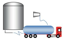
The liquid will flow to the tank powered by the pressure of the air or gas flowing from the compressor. The site tank will be connected to the vehicle by flexible hose of sufficient diameter (usually 80mm -3"). The site tank's vapour will exit the tank to the atmosphere (possibly through a scrubber or Vapour-recovery-unit if installed). After discharge the vehicles' tank needs to be brought to atmospheric pressure before the vehicle can be allowed to exit the site.
